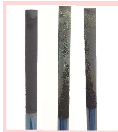
Deposits obtained in initial electrowinning tests
